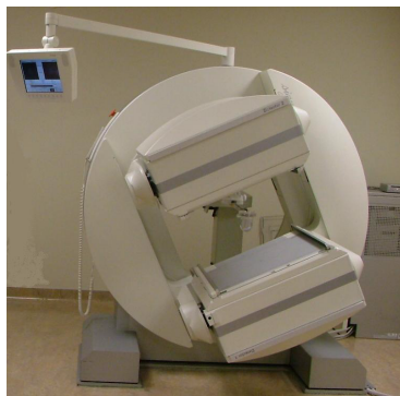
Fig. 1. A SPECT system that has two gamma cameras. A collimator is mounted on each camera. The two cameras rotate with the system gantry during data acquisition.
